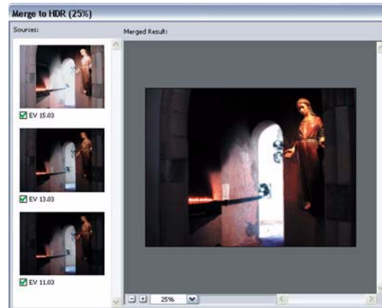
Use the Merge To HDR feature to combine three images shot with different exposures into a single picture.
